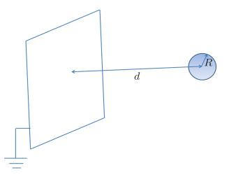
(a) Assume that the surface of the sphere is at a potential V. What is the potential in the interior of the sphere? What is the potential everywhere on the side of the plane that does not contain the sphere, i.e. to the left of the plane in the figure?
