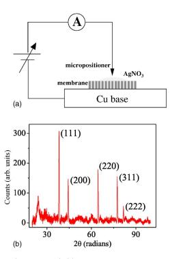
FIG. 1. (Color online) (a) A schematic of the setup used for making the nanowires. (b) XRD of 100 nm Ag wires. The peaks have been indexed to fcc Ag.
