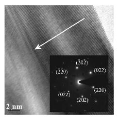
FIG. 3. HRTEM image of a 15 nm Ag wire. The arrow points out the twin boundary present in the sample. The inset shows the selective area diffraction pattern. The growth direction of the wires as seen from TEM is [100].
