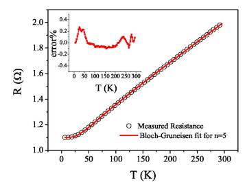
FIG. 6. (Color online) Fit to Bloch-Grüneisen formula [Eq. (1)] to the measured resistivity data for a 15 nm Ag wire. The inset shows the fit error (for definition see text) for n=5.
