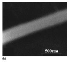
FIG. 2. SEM image of (a) 100 nm Ag wires taken after dissolving off the template in dichloromethane and (b) a single 200 nm Ag wire.
