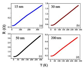
FIG. 5. (Color online) Resistance of arrays of Cu wires of diameter (a) 15, (b) 30, (c) 50, and (d) 200 nm.
