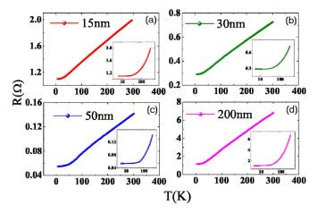
FIG. 4. (Color online) Resistance of arrays of Ag wires of diameter (a) 15, (b) 30, (c) 50, and (d) 200 nm. The inset shows the resistance with the temperature axis in a logarithmic scale in order to show more clearly the low-temperature behavior of the resistance.
